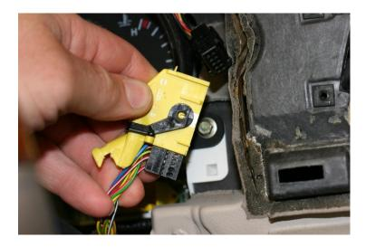
27. Note that the pin number for each corner pin (1, 13, 14, 26) is embossed in the black connector body. Using these corner numbers as a reference, separate out the <a href="RED/WHITE">CRANGE/YELLOW</a> wire at **pin #19** from the rest of the bundle. Then separate out the <a href="RED/WHITE">RED/WHITE</a> at **pin #3** from the rest of the bundle.
