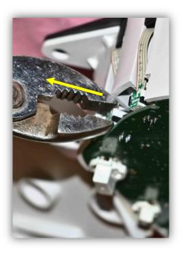
10. Fold this ribbon cable and connector end out of the case and replace the rear white cover of the instrument cluster and the six T-20 torx screws.
