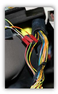
28. Use a tie wrap to strain relief the connections. Rewrap the lacing tape around the harness and then replace the foam around the harness. Secure it with the original fabric tape, wrapping the ends with electrical tape. If the original foam is badly deteriorated, self-adhesive weather-strip foam from any hardware store can be substituted.
