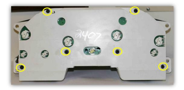
8. Remove the white back cover, opening from the right like a book to try to avoid tearing the identifying label on the left side, if possible. This will expose the circuit board. See below:
