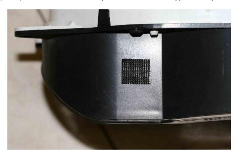
12. Install the RealGauge computer module on the Velcro with the label facing front. Align the left end with the curvature inflection point. The back end should be flush against the black plastic, and wedged under the white plastic protrusion.
