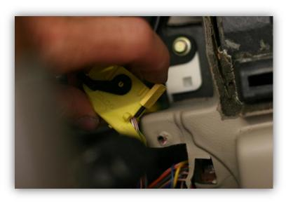
25. Starting about **3.5**" back from where the wires exit the connector, tap the **RED/WHITE** instrument cluster **right** connector wire with a *small Red/Black* Positap. Then connect the **RED/WHITE** wire from the RealGauge harness.
