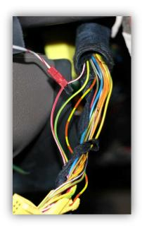
26. Next tap the YELLOW/GREEN instrument cluster **right** connector wire with a *small Red/Black* PosiTap. Then connect the YELLOW/GREEN wire from the RealGauge harness.
