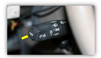
After about four seconds another test sequence should initiate and **you should release the button**. The coolant gauge needle should swing to the top of the scale, the alarm will go off briefly while it hits the red area, and then the needle will return to the low end of the scale. You should then hear four quick beeps in a sequence.
