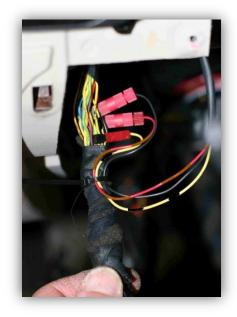
If the black shell was removed in step 18, replace it, and snap on the black hood retainer (from the end) and replace the zip tie.
