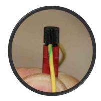
If a Posi-Tap is accidently not put on squarely, check the internal pin for breakage or bending prior to reuse. If one gets damaged, use the spare *Red/Black* Posi-Tap provided in the kit.
