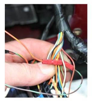
**Step 11:** Locate the heavy **brown** wire on the **BLUE** door module connector. If necessary peel back the electrical tape in the harness. Tap this wire with a **large blue** Posi-tap. Connect the <u>solid brown</u> wire from the remote top module wiring harness to this Posi-tap.
