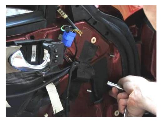
**Step 6:** Carefully extract the driver door module from the inside of the door cavity with the attached cables through the speaker opening. Make sure you do not lose the foam gasket inside the door. Carefully unravel about an inch of the electrical tape wrapping each of the harnesses near the connector. There is no need to unplug the connectors.
