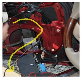
**Step 10:** Locate the **brown/green** wire on the **BLACK** door module connector. If necessary peel back the electrical tape in the harness. Tap the wire with a **small solid red** Posi-tap. Connect the **brown/green** wire from the remote top module wiring harness to this Posi-tap. Take care not to cross-thread the caps, particularly on these **small solid red** Posi-taps,.
