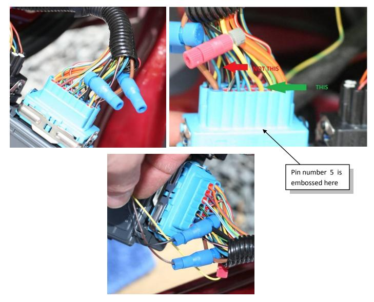
**Step 12:** Open the driver door fully. Turn the knurled plastic connector between the door and body harness counterclockwise to until the connector disengages. Remove the harness grommet end from the body and rotate it as shown below, with the connector facing outward:
