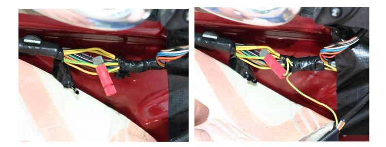
**Step 9:** Thread the two wires at the end of the remote module harness through the bottom of the driver door module opening and down through the speaker opening. Pull the remote module harness its full length through the speaker opening.
