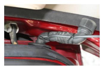
**Step 17:** Cutoff the tie wrap tails. Take the loose end of the cable and stuff the remaining cable through the adjacent open cavity of the front fender (it will be retrieved later). Reinsert the grommet in the door, and rotate the boot back to its original position. Re-insert the round connector into the body with a clockwise turn until it stops. The final product should look like the photo below, with the new cable tie wrapped behind the boot and barely visible:
