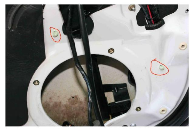
**Step 5:** Remove the three 7mm bolts retaining the Driver Door Module behind the sheet metal of the inner door.
