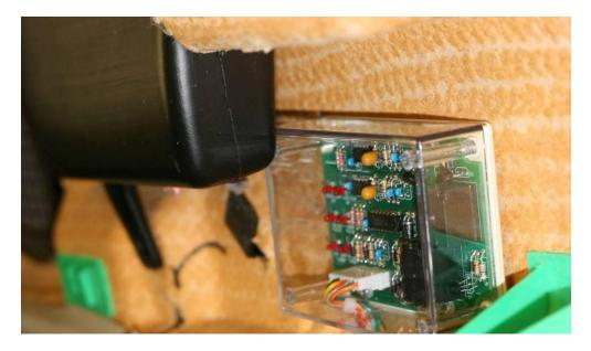
**Step 30:** Reinstall the puddle lamp connector. Reassemble the door panel trim and hardware on the door per the video instructions referenced above. Take care that the cable from the remote module remains within the door panel and does not protrude from the bottom of the door.
