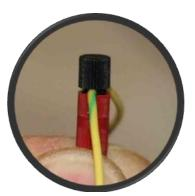
If a Posi-Tap is accidently not put on squarely, check the internal pin for breakage or bending prior to reuse.
