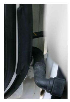
**Step 13:** Carefully pierce the rubber boot precisely as shown in the photo below with awl or sharp nail. Be careful not to damage wires in the boot.
