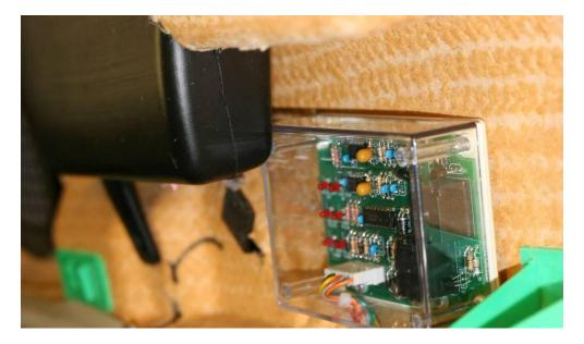
**Step 30:** Reinstall the puddle lamp connector. Reassemble the door panel trim and hardware on the door per the video instructions referenced above. Take care that the cable from the remote module remains within the door panel and does not protrude from the bottom of the door.
