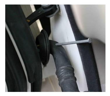
**Step 14:** Thread the two wires (white/red and blue/slate) into the eye of the supplied plastic needle. Use the needle to then pass the wires through the piecing in the rubber boot from the inside to the outside. Then pull the wire harness through the rubber boot by the outer black cable sheath (not the inner conductors). The final result should look like the picture below. <u>Be</u> sure to leave a few inches of cable slack inside of the door. Remove and discard the needle.
