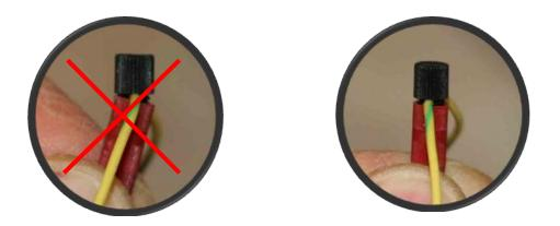
If a Posi-Tap is accidently not put on squarely, check the internal pin for breakage or bending prior to reuse.
