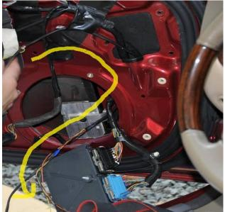
**Step 10:** Locate the **orange/blue** wire on the **BLACK** door module connector. If necessary peel back the electrical tape in the harness. Tap the wire with a **small solid red** Posi-tap. Connect the **orange/blue** wire from the remote top module wiring harness to this Posi-tap. Take care not to cross-thread the caps, particularly on these **small solid red** Posi-taps,.
