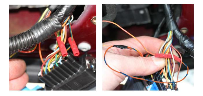
**Step 11:** Locate the heavy **brown** wire on the **BLUE** door module connector. If necessary peel back the electrical tape in the harness. Tap this wire with a **large blue** Posi-tap. Connect the <u>solid brown</u> wire from the remote top module wiring harness to this Posi-tap.
