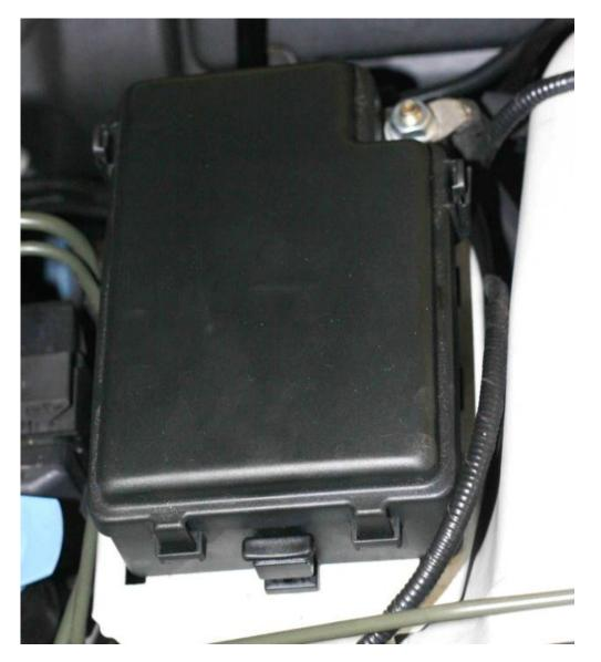
**Step 24:** Tilt up the fusebox, exposing the blue and black connectors on the underside. Route the harness from the wheel well to the fusebox and up through the opening underneath it.
