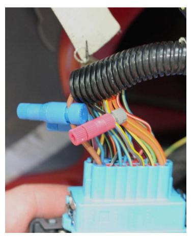
**Step 12:** Open the driver door fully. Turn the knurled plastic connector between the door and body harness counterclockwise to until the connector disengages. Remove the harness grommet end from the body and rotate it as shown below, with the connector facing outward:
