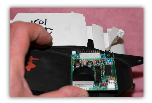
13. Twist the ribbon cable 180 degrees and plug it into the computer module as shown. Press firmly to seat it.
