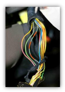
26. Starting about **3.5"** back from where the wires exit the connector, tap the PINK/YELLOW (may also be PURPLE-YELLOW) instrument cluster **right** connector wire with a *small Red/Black* Positap. Then connect the PINK/YELLOW wire from the RealGauge harness.
