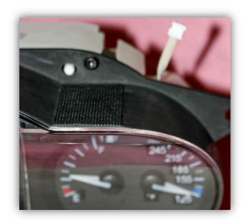
12. Install the RealGauge computer module on the Velcro with the label facing front. Align the left end with the curvature inflection point. The back end should be flush against the black plastic, and wedged under the white plastic protrusion.
