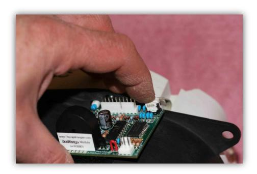
14. Plug the 10-position white connector from the RealGauge wiring harness into the computer module as shown. Make sure the stops on each end of the connector face towards the front of the instrument cluster. Seat the connector fully.
