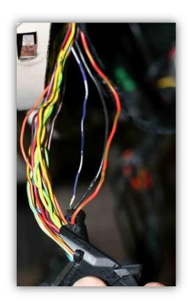
19. Starting about **3.5**" from where the wires exits the connector, tap the **BLACK** instrument cluster **left** connector wire with a *large Red/Slate* Positap. Then connect the **BLACK** wire from the RealGauge harness.
