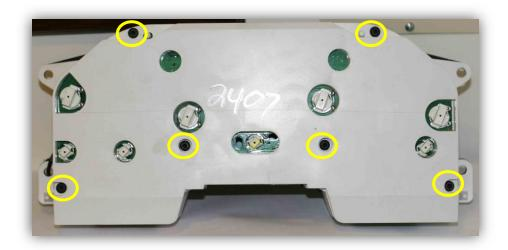
8. Remove the white back cover. This will expose the circuit board. See below:
