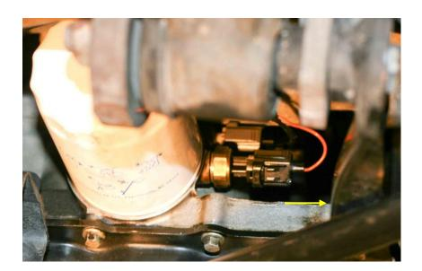
4. Remove the oil pressure switch using a 13/16" or 21mm deep socket. Have a basin or jar ready to catch the drips. Expect about 2 to 4 oz. of engine oil to drip out. Clean the mating surface on the engine block. Protective rubber gloves are recommended for this step.
