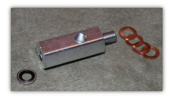
Finally, there is an easy solution to adding an aftermarket oil pressure gauge to a Jaguar V8. Fitting an oil pressure gauge had been a challenge due to the unusual M10 x 1.25 sensor fitting on Jaguar 4.0 and 4.2 liter V8 engines.
