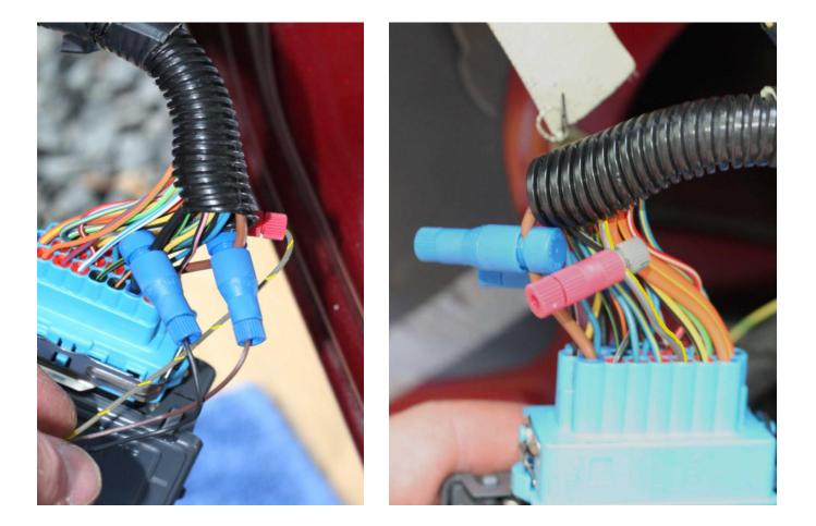
**Step 12:** Open the driver door fully. Turn the knurled plastic connector between the door and body harness counterclockwise to until the connector disengages. Remove the harness grommet end from the body and rotate it as shown below, with the connector facing outward:
