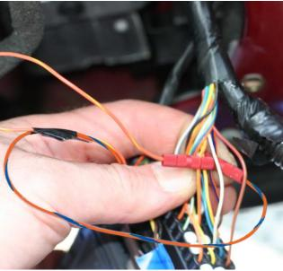
**Step 11:** Locate the heavy **brown** wire on the **BLUE** door module connector. If necessary peel back the electrical tape in the harness. Tap this wire with a **large blue** Posi-tap. Connect the <u>solid brown</u> wire from the remote top module wiring harness to this Posi-tap.
