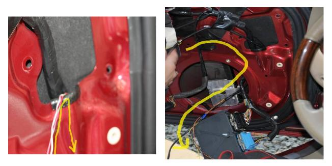
**Step 10:** Locate the **orange/blue** wire on the **BLACK** door module connector. If necessary peel back the electrical tape in the harness. Tap the wire with a **small solid red** Posi-tap. Connect the **orange/blue** wire from the remote top module wiring harness to this Posi-tap. Take care not to cross-thread the caps, particularly on these **small solid red** Posi-taps,.
