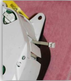
11. Place the instrument cluster with the top facing you. Using an alcohol pad, clean the black plastic surface above the gas gauge and above the tachometer area on top of the cluster and let it dry. Mount the 1" x 2" self-adhesive Velcro strip over the fuel gauge along the curvature inflection line, as shown below.
