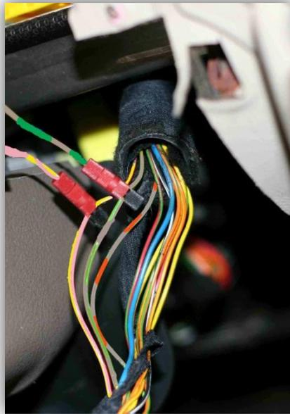
28. Next tap the **ORANGE/SLATE** wire on **pin 19** of the instrument cluster **right** connector with a *small Red/Black* Posi-Tap. Then connect the **ORANGE/SLATE** wire from the RealGauge harness (note that the SLATE stripe on the RealGauge harness **ORANGE/SLATE** wire may be very faint).
