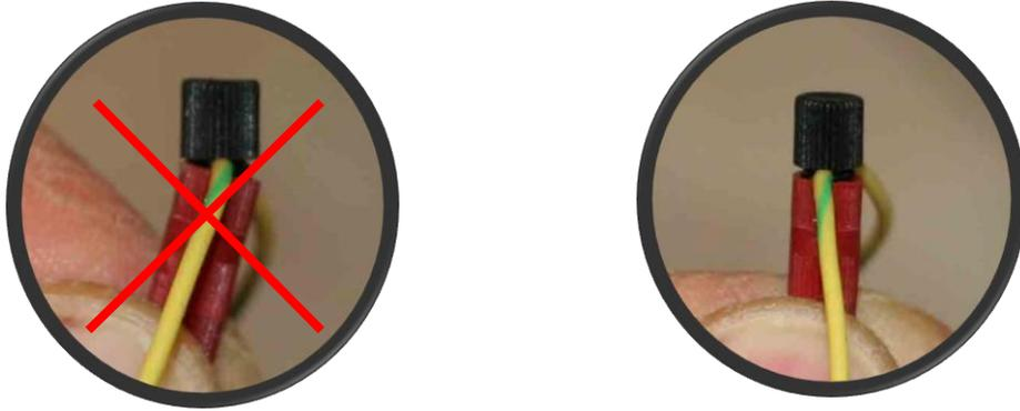
If a Posi-Tap is accidentally not put on squarely, check the internal pin for breakage or bending prior to reuse. If one gets damaged, use the spare **Red/Black** Posi-Tap provided in the kit.
