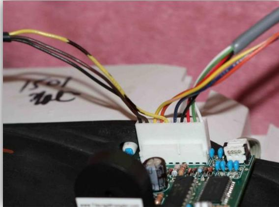
15. With the harness cables hanging on the right and left sides from the last step, replace the instrument cluster in the vehicle by tilting the bottom in place first. **Be sure the harness cables remain in front of the four mounting brackets. Do not** plug the two instrument cluster connectors back in at this time. Press down on the RealGauge module slightly, if necessary, to clear the dash opening while you rotate the upper part of the cluster into the opening.
