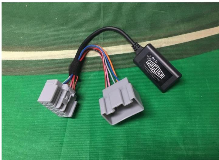
Our Bluetooth Streaming Adaptor is a lower-cost and simpler alternative to the ACM, providing a Bluetooth link between your phone and the car radio, through the AUX input. It is necessary for a Jaguar dealer to enable the AUX input, same as if fitting an ACM, then you can plug in this adaptor harness.
