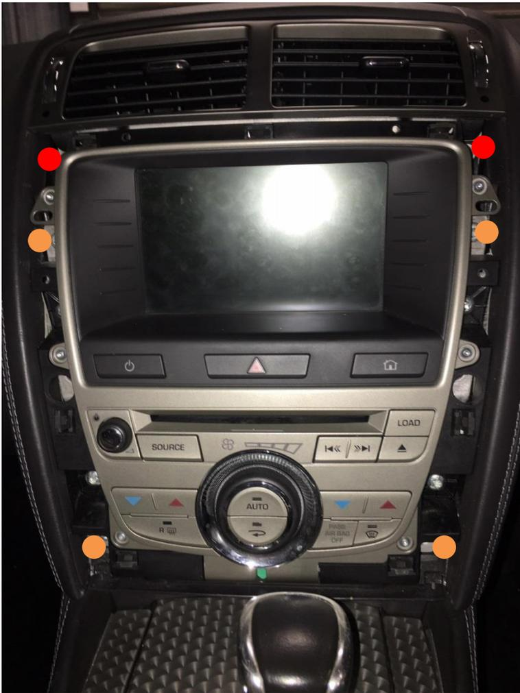
Remove the veneer trim from around the screen and audio/climate panel with a suitable trim removal tool.
