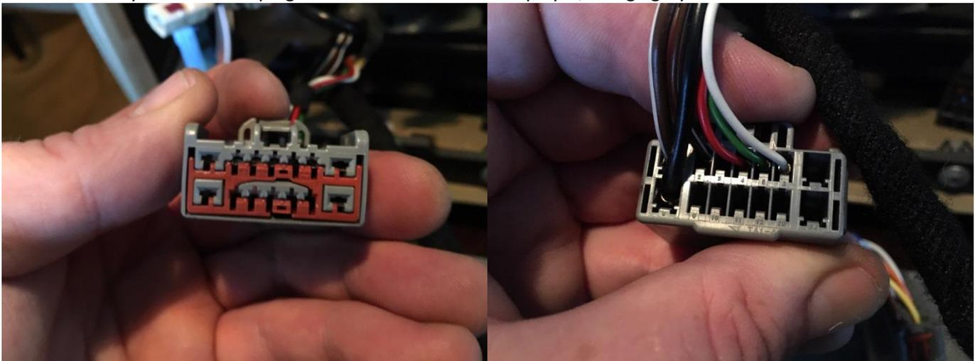
Insert this male connector taken out of the CD player into the female connector of the adaptor harness. Insert the male connector of the adaptor harness into the back of the CD player.
