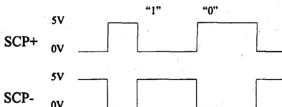
The link is used as a star network (see figure E). There is no controlling module, a system of non-destructive arbitration & message priorities is used to determine access to the bus. The format of these messages is pre-defined and is controlled by a standardised Ford world-wide data-base.
