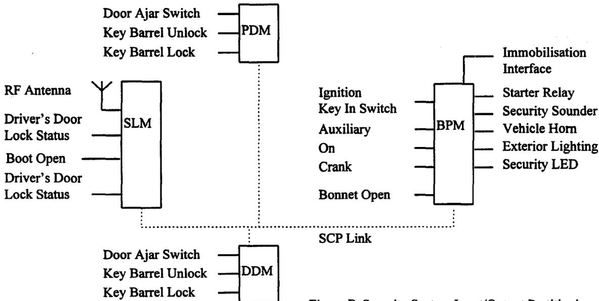
Figure F: Security System Input/Output Partitioning
