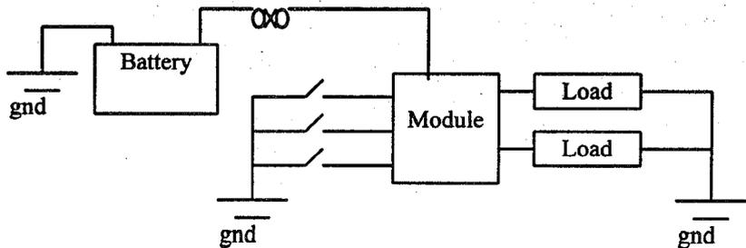
The addition of a multiplexed link between these modules allows information to be shared whilst REDUCING the number of harness wires required (see figure F, later in paper). Once a switch or load is wired to one module, the status or control of that wire is available to all the other modules on the network via the multiplexed link.
