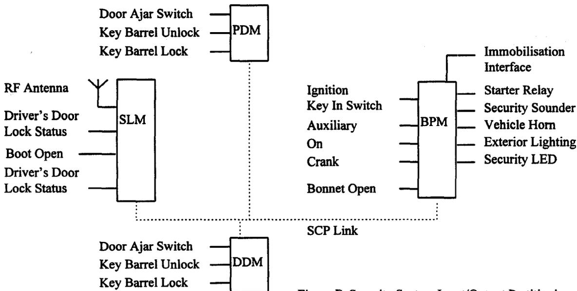
Figure F: Security System Input/Output Partitioning
