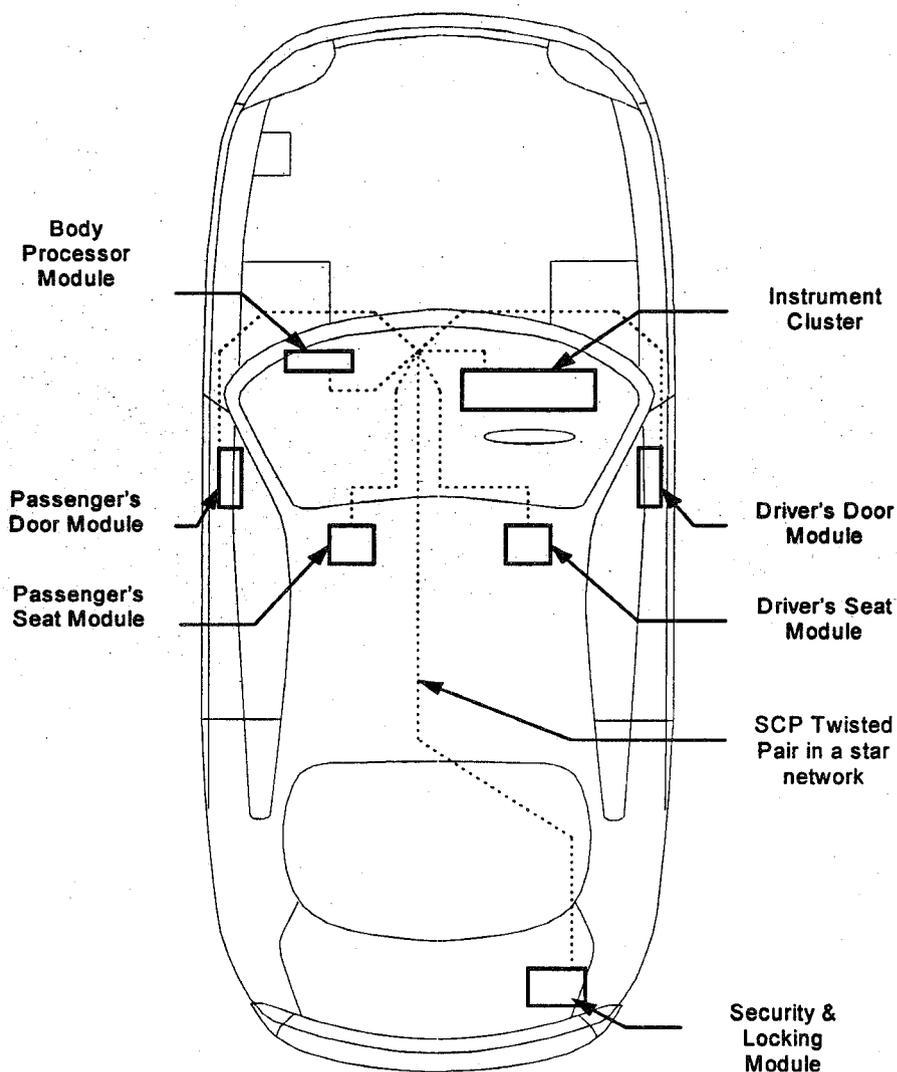
Figure E: Body System Module Location
