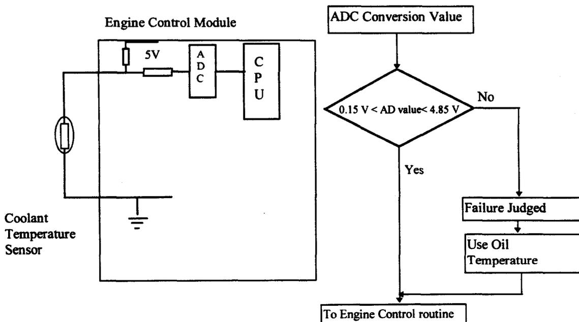
Additional sensor faults also diagnosed include 'stuck at' faults where for example the air temperature sensor resistance could stick giving a constant temperature reading of 100°C. These type of faults would not be diagnosed using the above method since the output voltage would fall inside the normal voltage range.
