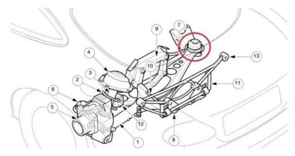
The XK8 rear suspension design shown in the line drawing above reduces the natural tendency of the car to squat under acceleration. Like the front end, the XK8 rear suspension utilizes a control-arm design, with the coil spring and damper combined into a single unit. The spring is seated directly on
