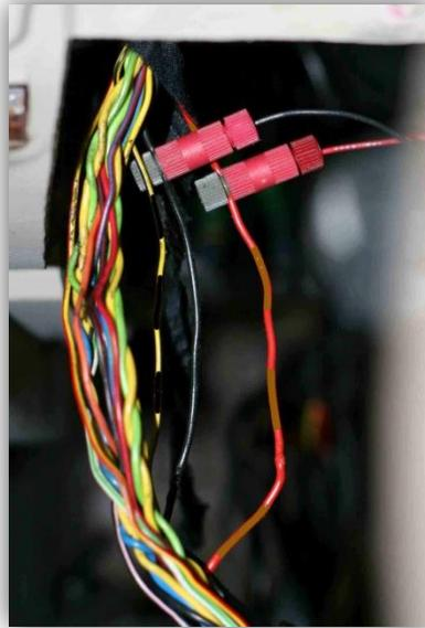
21. Next tap the **YELLOW/BLACK** instrument cluster **left** connector wire with a *small Red/Black* Posi-Tap. Then connect the **YELLOW/BLACK** wire from the RealGauge harness.
