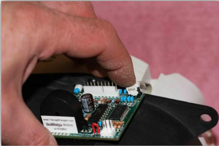
On XJ/X308 models, also mount the speaker over the tachometer on the Velcro as shown.
