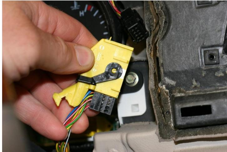
27. Note that the pin number for each corner pin (1, 13, 14, 26) is embossed in the black connector body. Using these corner numbers as a reference, separate out the **ORANGE/YELLOW** wire at **pin #19** from the rest of the bundle. Then separate out the **RED/WHITE** at **pin #3** from the rest of the bundle.
