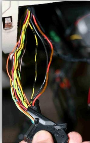
19. Starting about **3.5"** from where the wires exit the connector, tap the **BLACK** instrument cluster **left** connector wire with a *large Red/Slate* Positap. Then connect the **BLACK** wire from the RealGauge harness.
