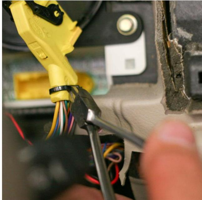
25. On the yellow connector, slide off the hood retainer on the end with your thumb. If it proves difficult, you can alternatively pry off the hood retainer from one side gently with a pair of pliers as shown.
