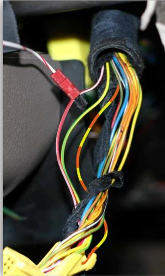
26. Next tap the **YELLOW/GREEN** instrument cluster **right** connector wire with a *small Red/Black* Posi-Tap. Then connect the **YELLOW/GREEN** wire from the RealGauge harness.
