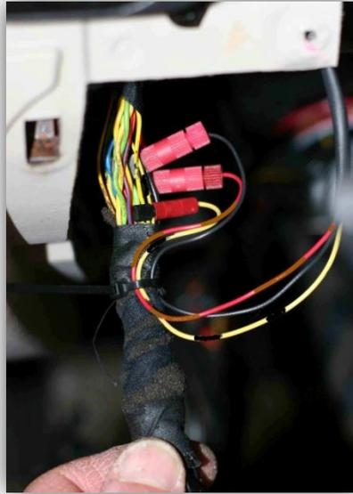
If the black shell was removed in step 18, replace it, and snap on the black hood retainer (from the end) and replace the zip tie.
