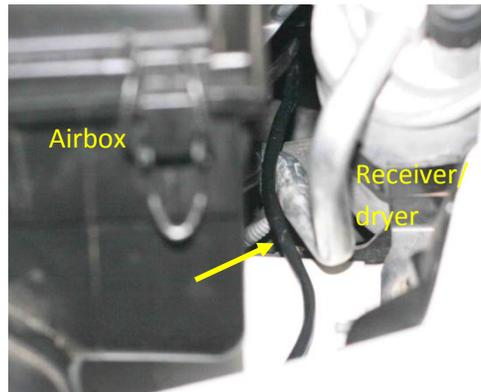
32. Route the sensor cable under the airbox snorkel and tie wrap it to the airbox bolt.
