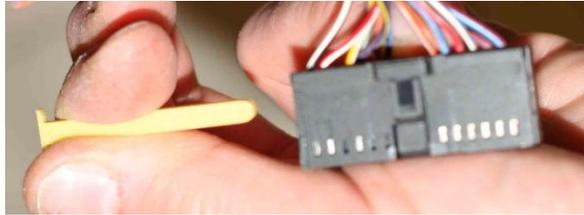
12. Note the tiny pin number references embossed in the corners of the connector face (you may need a bright light and a magnifier). They can be used to reference the other pin positions by counting.
