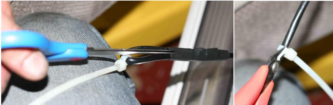
41. Route the sensor cable over kick panel mounting rail below the dashboard. Then route sensor cable up and alongside the left of the main instrument cluster and over the top of the cluster. Plug the sensor cable into the 3-pin connector on the front edge of the RealGauge module with the red wire on the left and the black wire on the right.
