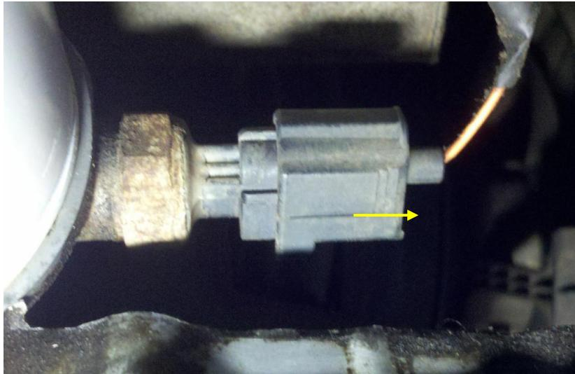
24. Remove the oil pressure switch using a 13/16" or 21mm deep socket. Have a basin or jar ready to catch the drips. Expect about 2 to 4 oz. of engine oil to drip out. Clean the mating surface on the engine block. Protective rubber gloves are recommended for this step.
