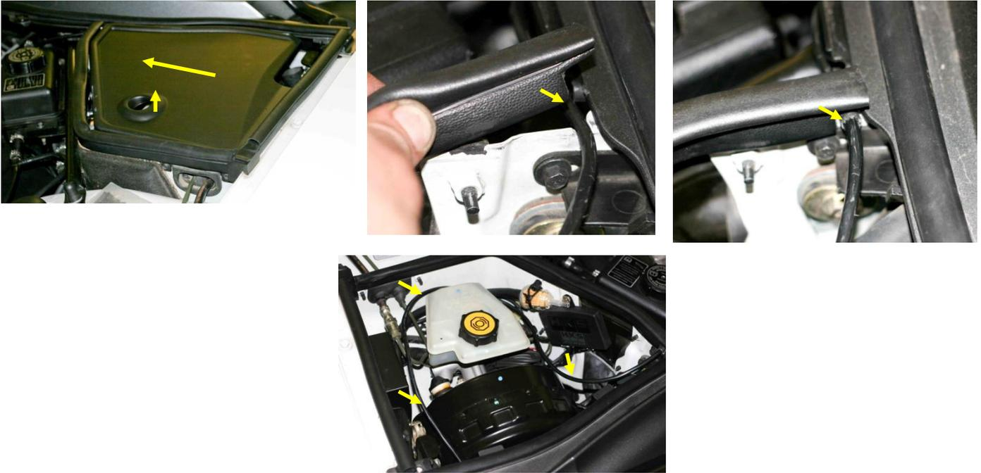
36. Pry loose the accordion rubber boot near the fender on the bottom of the brake booster compartment (see photo below). Use a flat blade screwdriver if necessary to assist. There may be a rubbery adhesive bond between the rubber and metal that you need to break. (It is not absolutely necessary, but if you have difficulty with this step remove the wipers and the plastic grille under the wipers and to gain easier access.)
