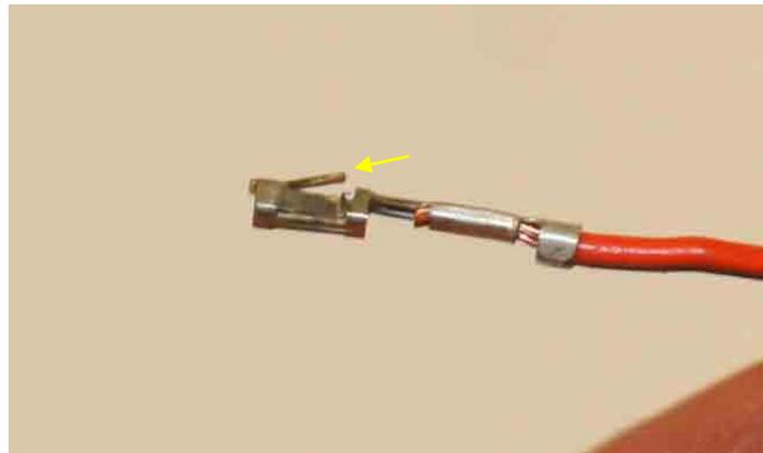
16. Insert the terminals into the four position connector body supplied in the kit. Hold the four pin connector with the large openings facing you, and the white plastic insert facing down as shown below. Position 1 is on the right, and position 4 is on the left. Terminals are inserted with the locking tab facing down with the connector body held as shown.
