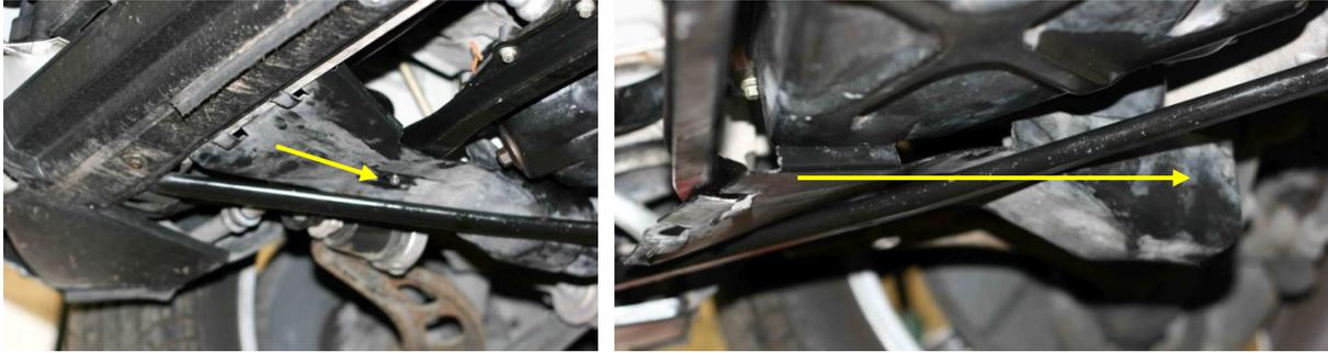
23. Squeeze the connector tab and unplug the connector from the oil pressure switch (the one with the orange wire) adjacent to the oil filter. If your car has another sensor with two wires (not all do), leave the other sensor alone.
