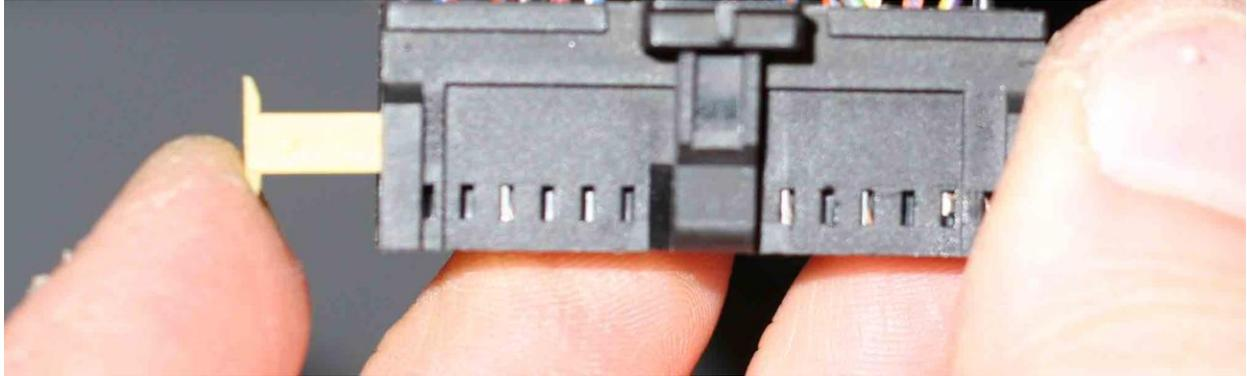
15. Check that the locking tab on each terminal stands out about 10 degrees, and gently bend it back into position if necessary.
