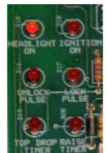
**h:** The door must still be locked. Press the headlight button on the remote key fob once. Then immediately press the UNLOCK button on the key fob. The top should drop! The red 'Drop Timer' LED should remain on for about 35 seconds. (The headlight LED will extinguish after about 25 seconds.)
