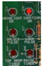
**d:** With the ignition on, lower the top from inside the car. Make sure you hear a 'ding' at the end of the cycle. Then raise the top from the inside of the car. If there is any malfunction, go back to step 27a and repeat again. If it works, go to the next step.
