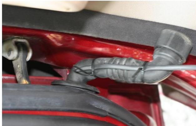
**Step 17:** Cutoff the tie wrap tails. Take the loose end of the cable and stuff the remaining cable through the adjacent open cavity of the front fender (it will be retrieved later). Reinsert the grommet in the door, and rotate the boot back to its original position. Re-insert the round connector into the body with a clockwise turn until it stops. The final product should look like the photo below, with the new cable tie wrapped behind the boot and barely visible:
