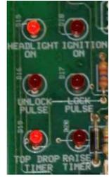
**i:** Now with the door unlocked, press the headlight button on the remote key fob once. Then immediately press the LOCK button on the key fob. The top should raise back up! The red 'Raise Timer' LED should remain on for about 35 seconds. (The headlight LED will extinguish after about 25 seconds.)
