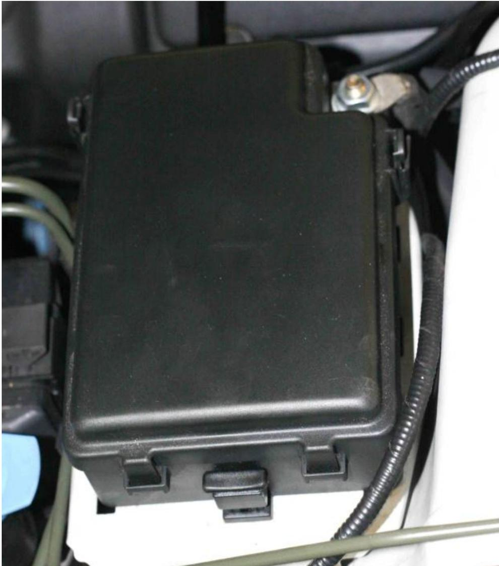
**Step 24:** Tilt up the fusebox, exposing the blue and black connectors on the underside. Route the harness from the wheel well to the fusebox and up through the opening underneath it.
