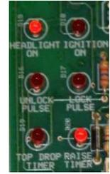
**j:** The door must still be locked. Press the headlight button on the remote key fob once. Then immediately press the UNLOCK button on the key fob. As the top drops hit the LOCK button midway during the cycle. If the headlights are still on, the cycle should reverse and the top will raise back up. If the headlights are off, the top motion should stop mid-cycle. To resume motion, hit the headlight button and hit LOCK or UNLOCK buttons.
