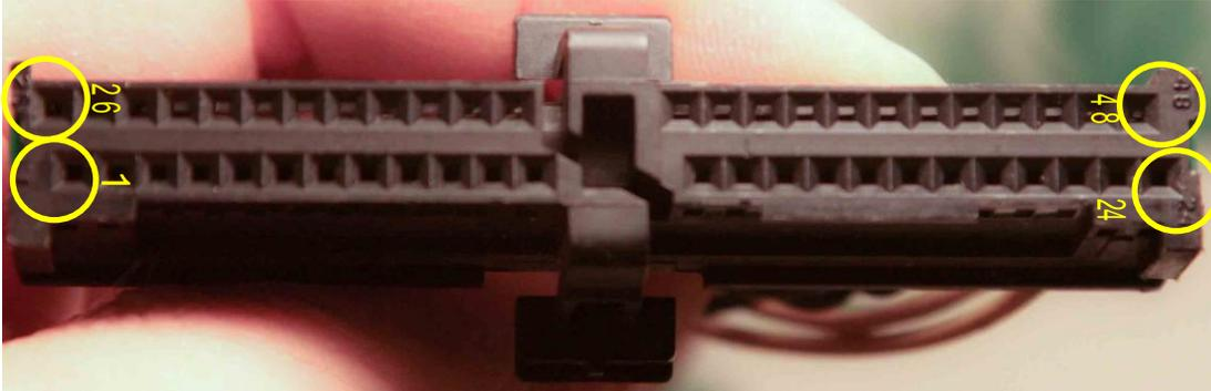
Sort through the instrument cluster **left** connector wires and separate out the **BLACK** (pin #26), **BROWN/RED** (pin # 25) and **SLATE/BLUE** (pin #10) wires from the rest of the bundle. (Note: The wires may have lengthwise color stripes instead of bands as in the photo).
