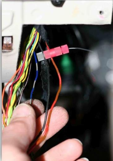
20. Next tap the **BROWN/RED** instrument cluster **left** connector wire with a *large Red/Slate* Posi-Tap. Then connect the **BROWN/RED** wire from the RealGauge harness.
