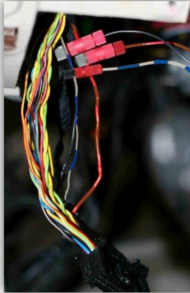
22. Use a tie wrap to strain relief the connections. Rewrap the lacing tape around the harness and then replace the foam or felt around the harness. Secure it with the original fabric tape, wrapping the ends with electrical tape. If the original foam or felt is badly deteriorated, self adhesive weather-strip foam from any hardware store can be substituted. The foam or felt is primarily used to prevent wire abrasions and rattles.
