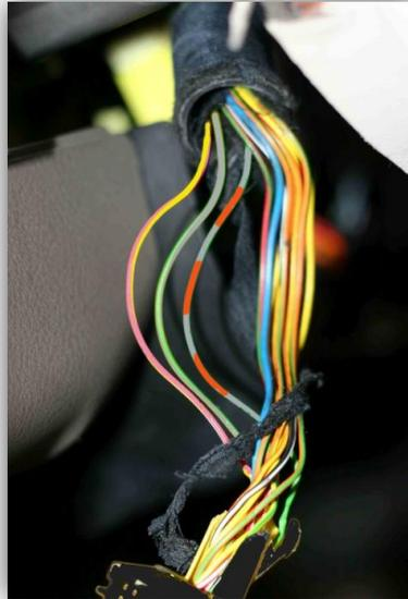
26. Starting about **3.5"** back from where the wires exit the connector, tap the **PINK/YELLOW** (may also be **PURPLE-YELLOW**) instrument cluster **right** connector wire with a *small Red/Black* Positap. Then connect the **PINK/YELLOW** wire from the RealGauge harness.
