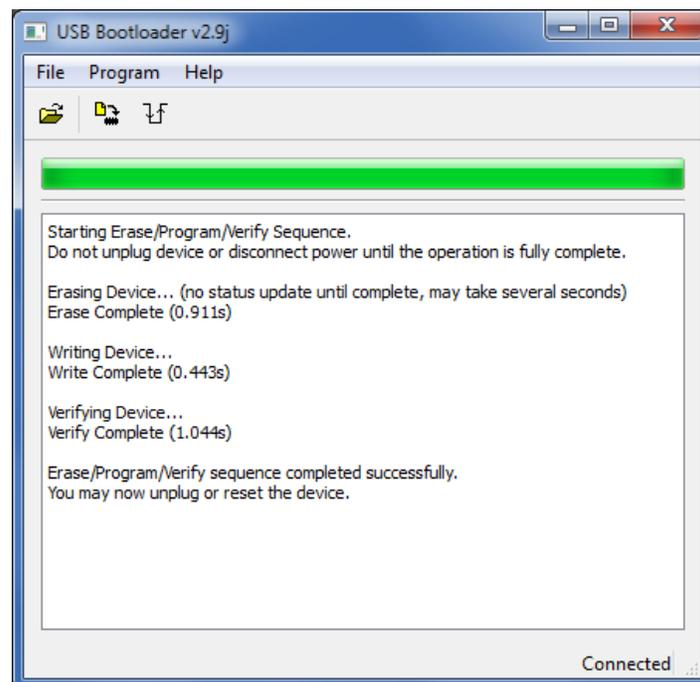
12. Click on the reset button, then IMMEDIATELY unplug the USB cable from the PC (you have up to 6 seconds between clicking on reset and unplugging the USB cable).
