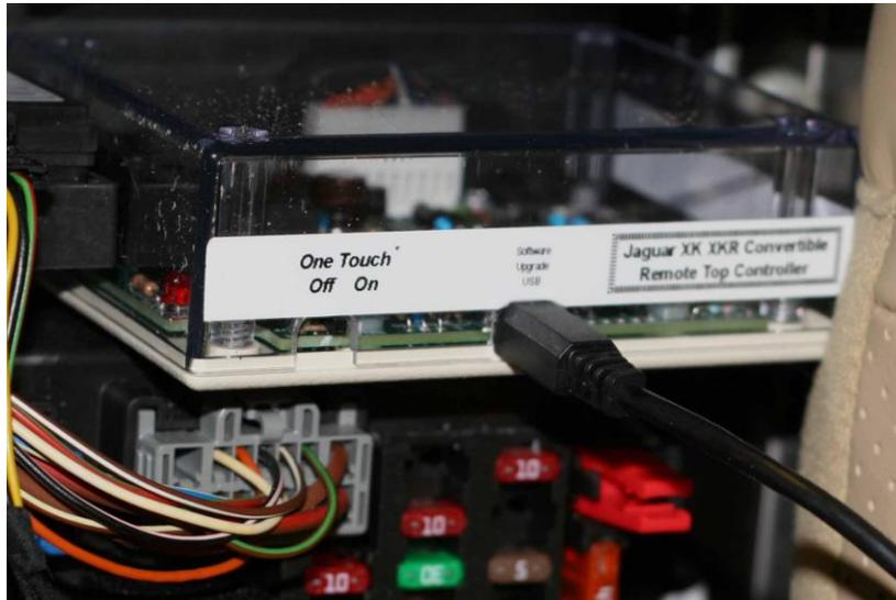
6. Turn on the ignition. Note that the two GREEN LEDs on the remote top module should be blinking rapidly.
