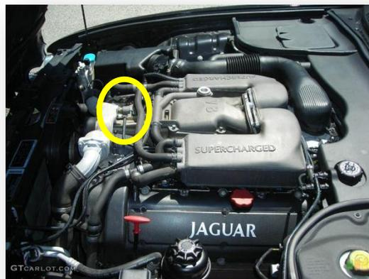
2. Plug each of the two wires from the variable resistor into a terminal in the coolant temperature connector shell (harness side). Either wire can go in either position. See below.
