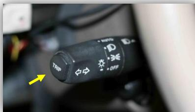
9. Adjust the variable resistor until the coolant temperature on your OBDII scanner reads 245 degrees F (or as close to it as you can get). Be aware that the radiator fans will cycle on spontaneously. This is normal. Then press and release the trip cycle button **only once**. You will hear a beep. Now the needle on the coolant gauge should have moved to 3/4 scale (215 degrees F).
