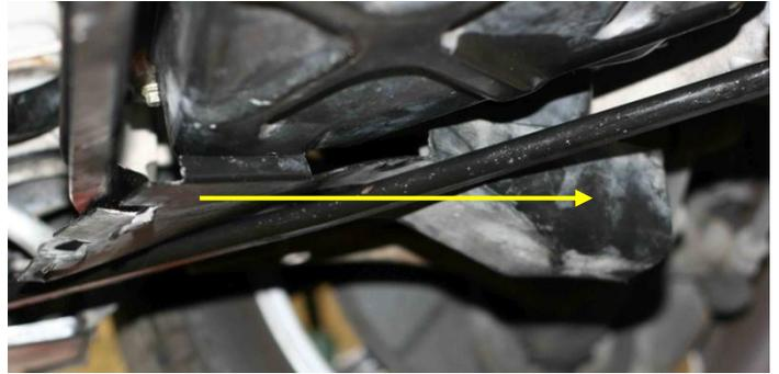
3. Squeeze the connector tab and unplug the connector from the oil pressure switch (the one with the single orange wire) adjacent to the oil filter. If your car has another sensor with two wires (not all do), leave the other sensor alone.
